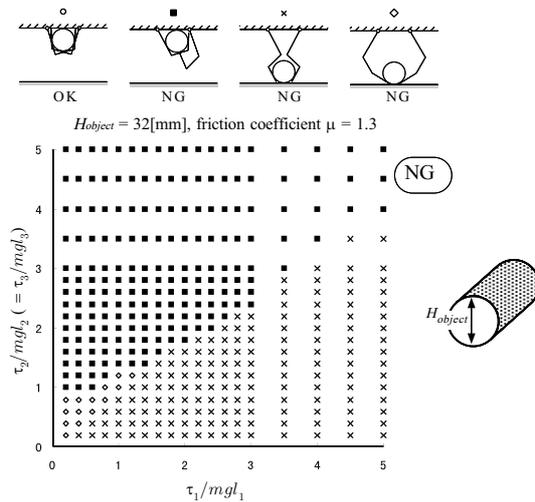
Fig. 12. Success map for a cylindrical object ( $\mu = 1.3$ ).
