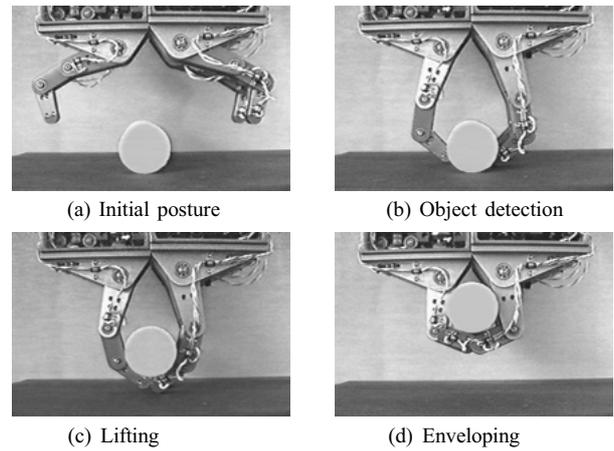
Fig. 10. Sliding based grasp.
